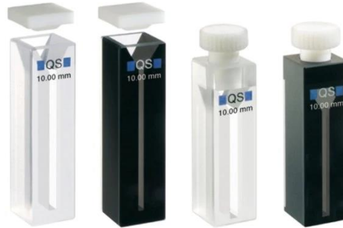
Semi micro cell, 1400 \mu L
